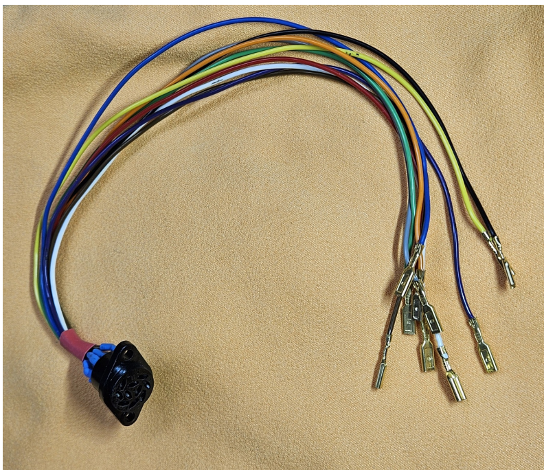
Photo 1 - Wiring harness of the external remote-control socket: these wires are no longer used.
